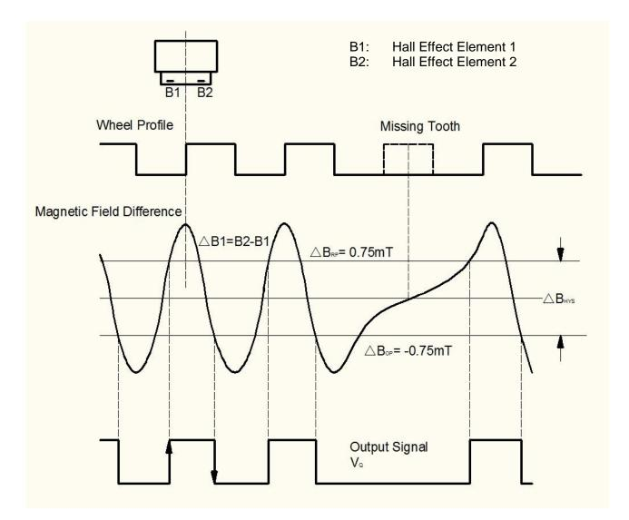
Operating point:B2-B1 <  $\Delta B_{OP}$  switches the output ON (V<sub>Q</sub> = LOW)Release point:B2-B1 >  $\Delta B_{RP}$  switches the output OFF (V<sub>Q</sub> = HIGH) $\Delta B_{RP} = \Delta B_{OP} + \Delta B_{HYS}$
