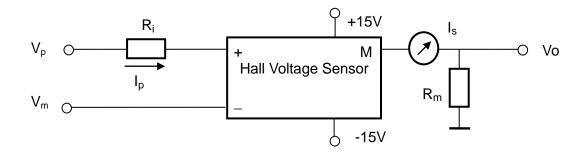
A magnetic field is generated by current  $I_p$  when a voltage  $(V_p-V_m)$  is applied on the input terminals of the sensor through the primary resistor  $R_i$ . This magnetic field is compensated with the reverse magnetic field caused by the current  $I_s$  in the secondary coil. The field compensation effect can be detected with a Hall Effect element. One obtains the following equation when the magnetic flux is zero:
