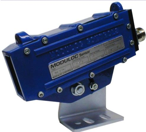
The self-contained Model MD8100 Hot Product Detector is available with either air coolant chamber venting as air purge or alternatively with a water coolant chamber and separate air purge.
