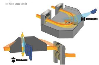
Being an intelligent digital device, the Trailfinder's response time may be precisely set to accommodate black spots, steam/water or hot scale in its field of view without detriment to its performance. Detects the product edge precisely and repeatability regardless of the product size and changes in temperature.
