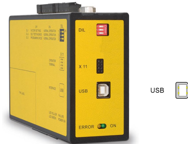
Figure 30 - [USB] type B USB port
