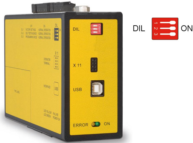
Figure 28 - [S1] 3-position DIP switch
